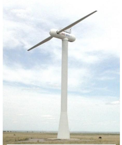
600 kW utility-scale Advanced Research Turbine at NREL's National Wind Technology Center near Golden, CO, USA. Note how the variable-pitch blades are positioned so they can't make power—the0 turbine is shut down and can't spin. Photo by the author.
