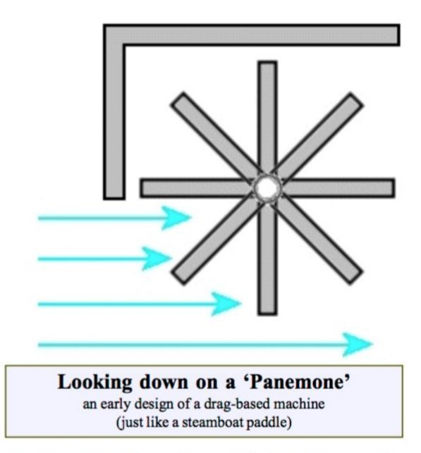
Note the wall that's erected around the half of the machine that is hurting performance by moving against the wind. In any drag-based design, the blades can never move faster than the wind. This turns out to be a critical concept for both efficiency and the ease of generating electrical power. Wheel can't move faster than the wind
