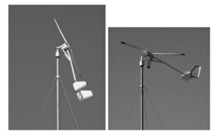
FIGURE 6.25 Rotor axis offset from horizontal pivot point for control. Left: run position at wind speeds below 13 m/sec. Right: furled position in high winds.
