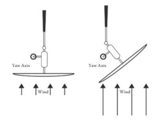
FIGURE 6.24 Furling diagram of rotor axis offset from tower (yaw axis) with hinged tail.
