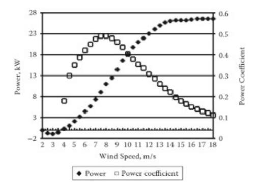
FIGURE 6.13 Experimental power and power coefficient for a Carter 25 rated 25 kW, 10 m in diameter. At 3 m/sec, the turbine uses power (energy for field coils of induction generator).
