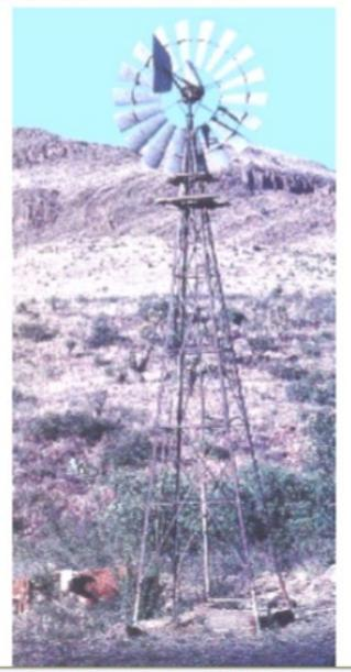
A typical Aermotor water pumping windmill, still common and in operation all over the American West. Photo courtesy of DeanBennett.com, Denver, CO. This company sells all the replacement parts to keep these beautiful old machines running, and also sells new waterpumping windmills. Drag based horizontal wind turbine
