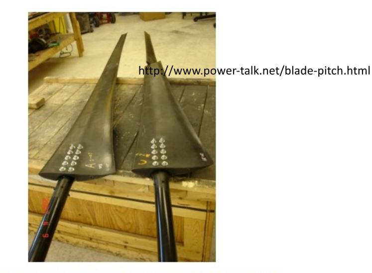
Blade tip pitch is another variation that is used on one small turbine made in the U.S. It is the machine built by the Ventera Energy Corporation. The outer tip of the blade responds to centrifugal force instead of the whole blade.
