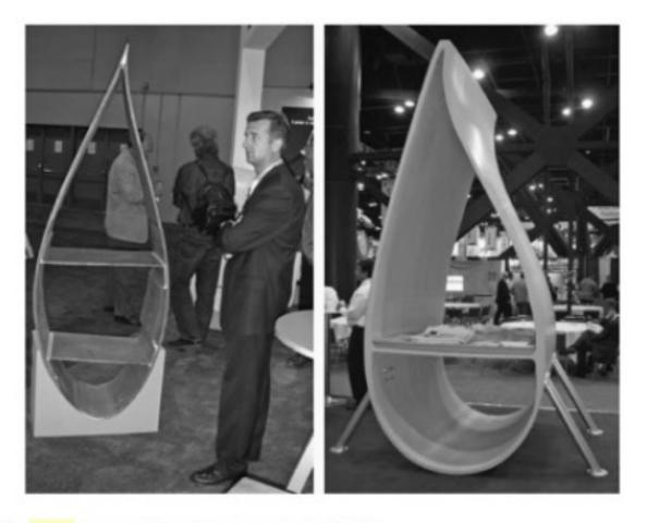
FIGURE 6.17 Blade cross sections for megawatt wind turbine.
