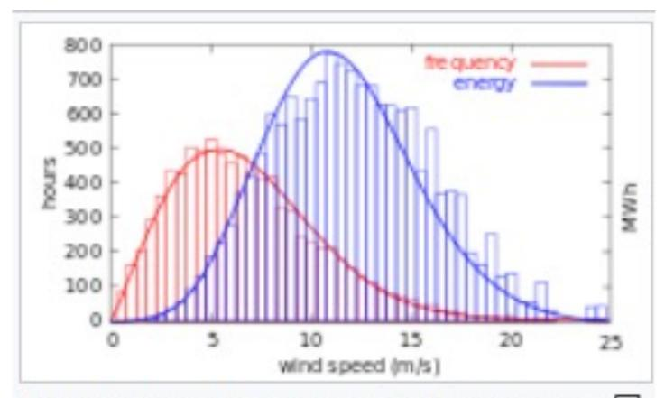
Distribution of wind speed (red) and energy generated (blue). The histogram shows measured data, while the curve is the Rayleigh model distribution for the same average wind speed.
