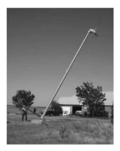
FIGURE 6.18 Small (1.8 kW) wind turbine mounted on-10 m pole tower, no guy wires, with gin pole. Note sweep blades.
