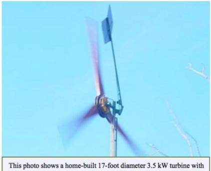
This photo shows a home-built 17-foot diameter 3.5 kW turbine with the tail in fully furled position. The machine is still making near maximum power, but it facing at an angle into the wind to reduce wind input. Photo by Dan Bartmann.
